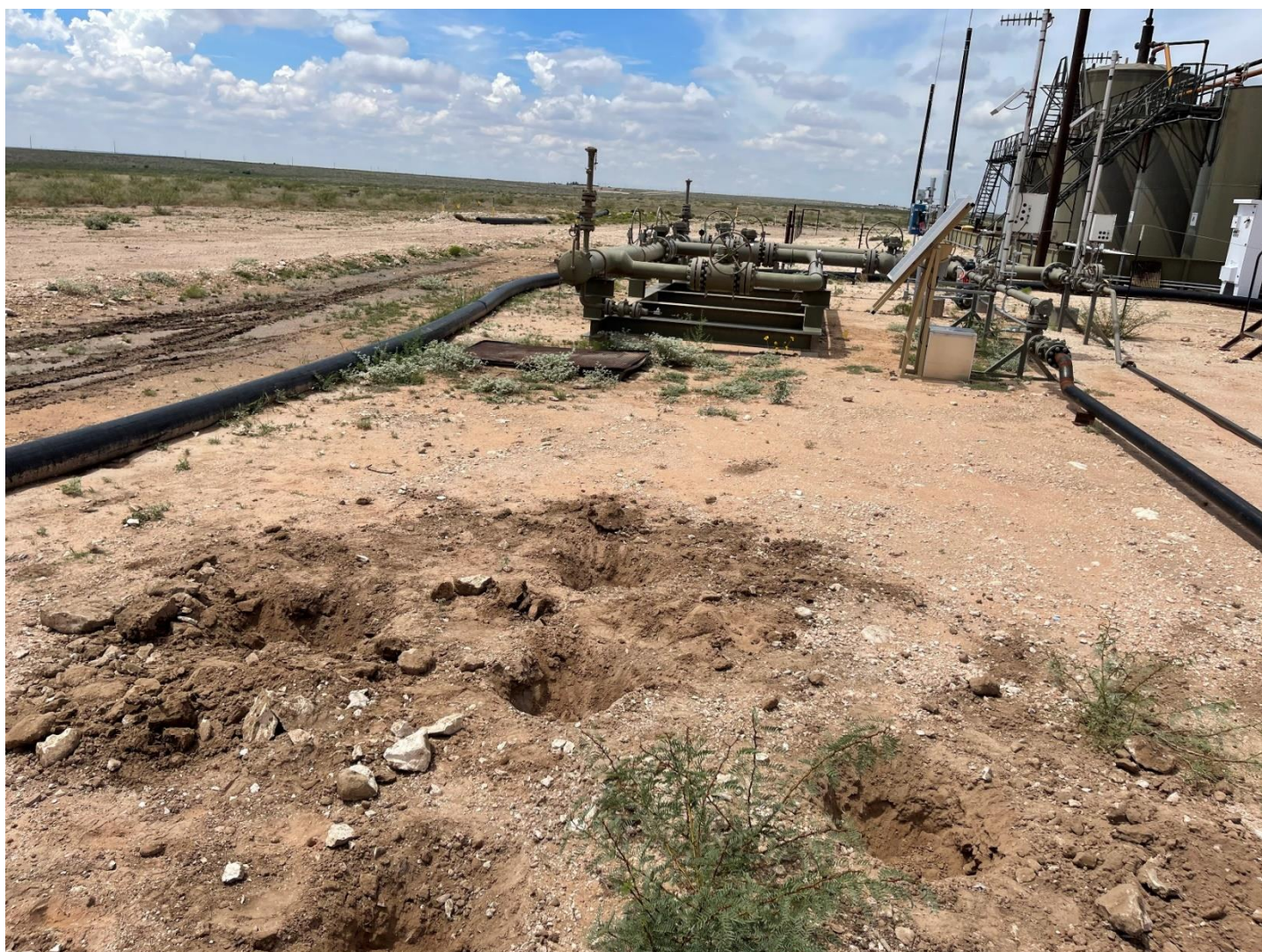
Image 11: Collection of Composite Samples in Quadrant A2. Quadrants A1 and A3-A10 were Collected in Similar Fashion
