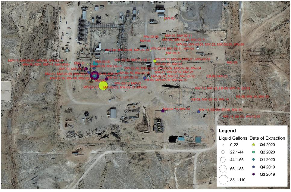
Note: Extractions from multiple wells are depicted at the center point between these wells (the midpoint between MW-03 and MW-02-11, for example).
