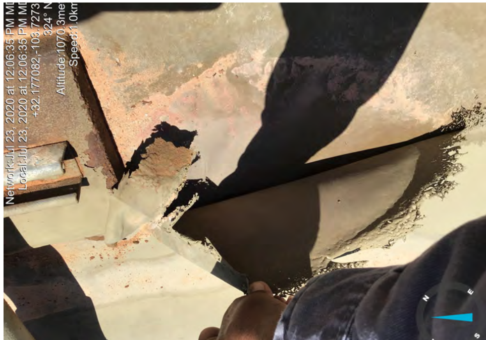
East side, inside pump#3, liner patch unglued
