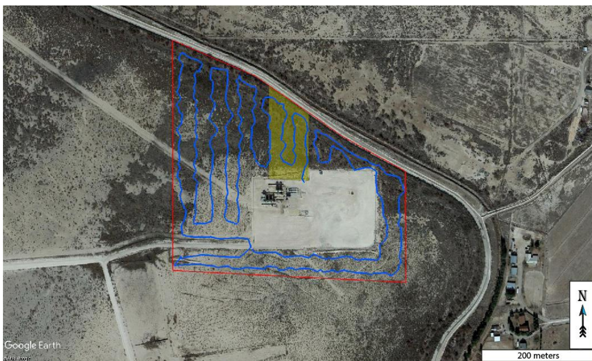
Figure 4: Survey overview. Red polygon is the study area. Transparent yellow area is the approximate spill location. Blue wavy lines are the actual survey lines. Background image credit: Google Earth. Image date: December 21, 2019. Datum: WGS-84.
