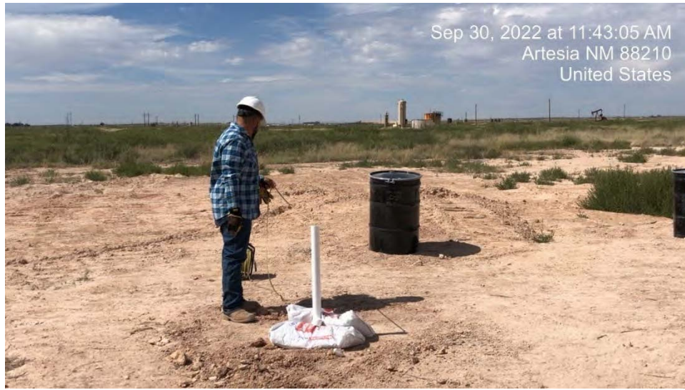
PHOTOGRAPH NO. 3 – A typical view of the gauging of the temporary monitor wells.
