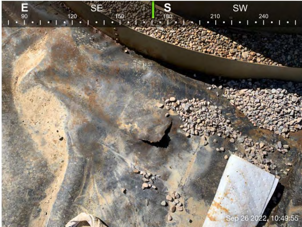
Photo 3: Hole in liner, 9/26/2022.
