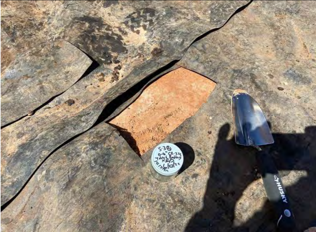
Photo 7: View of S-3 sample location. Holes in the liner were expanded for access and samples were collected directly beneath liner holes.
