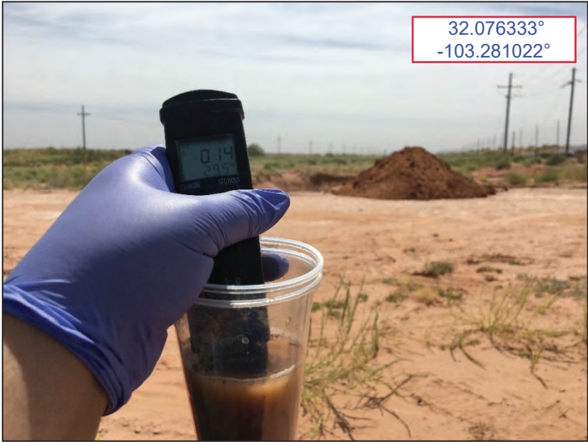
9-21-2021 Field test of imported fill; EC = 0.14 dS/m
