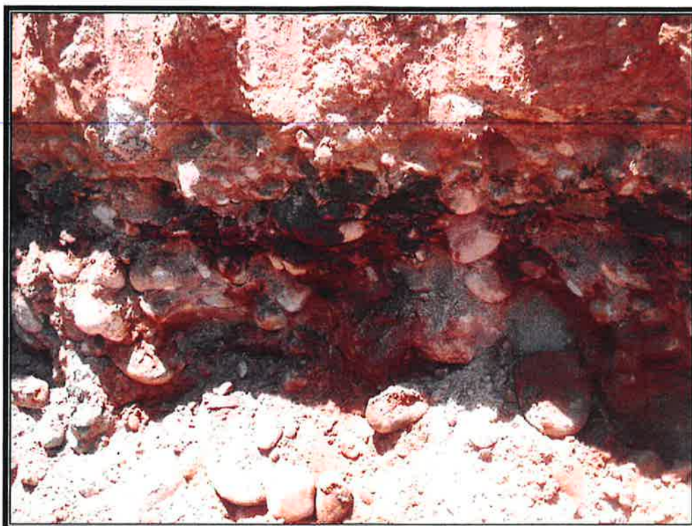
Photo 4: Visible Line of Contamination along the Walls
