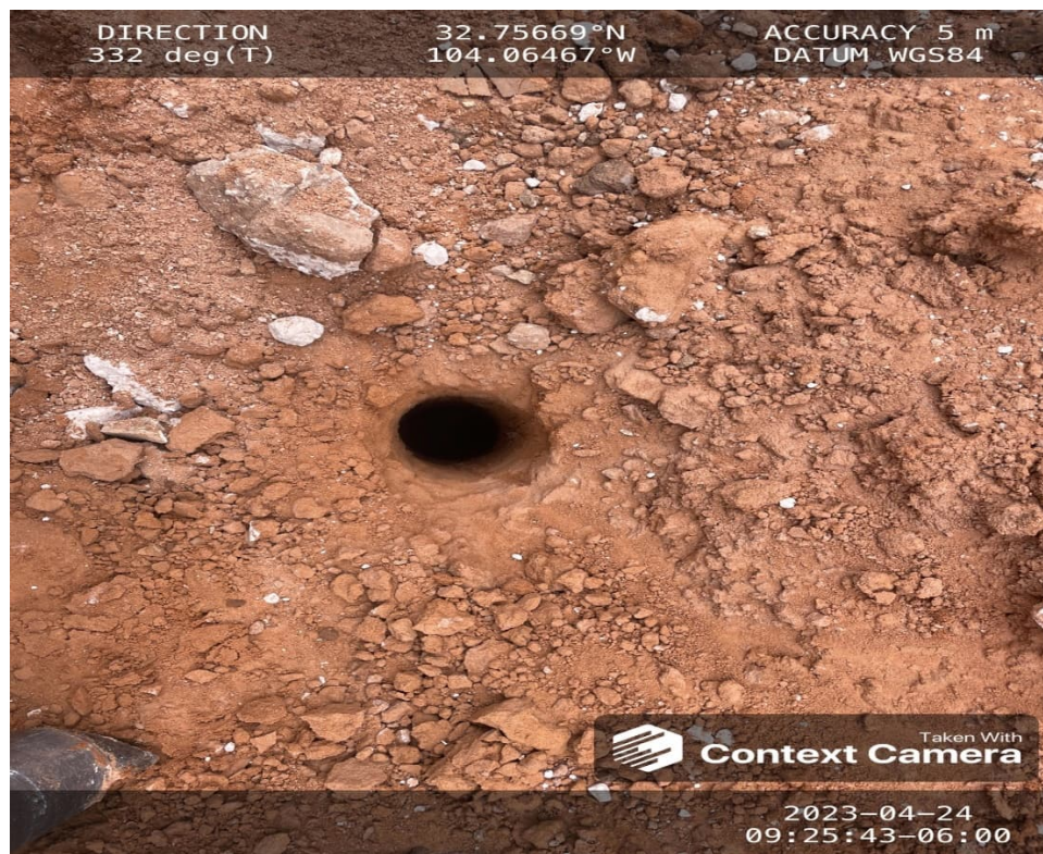
PHOTO 6: View of hand auger vertical floor delineation.
