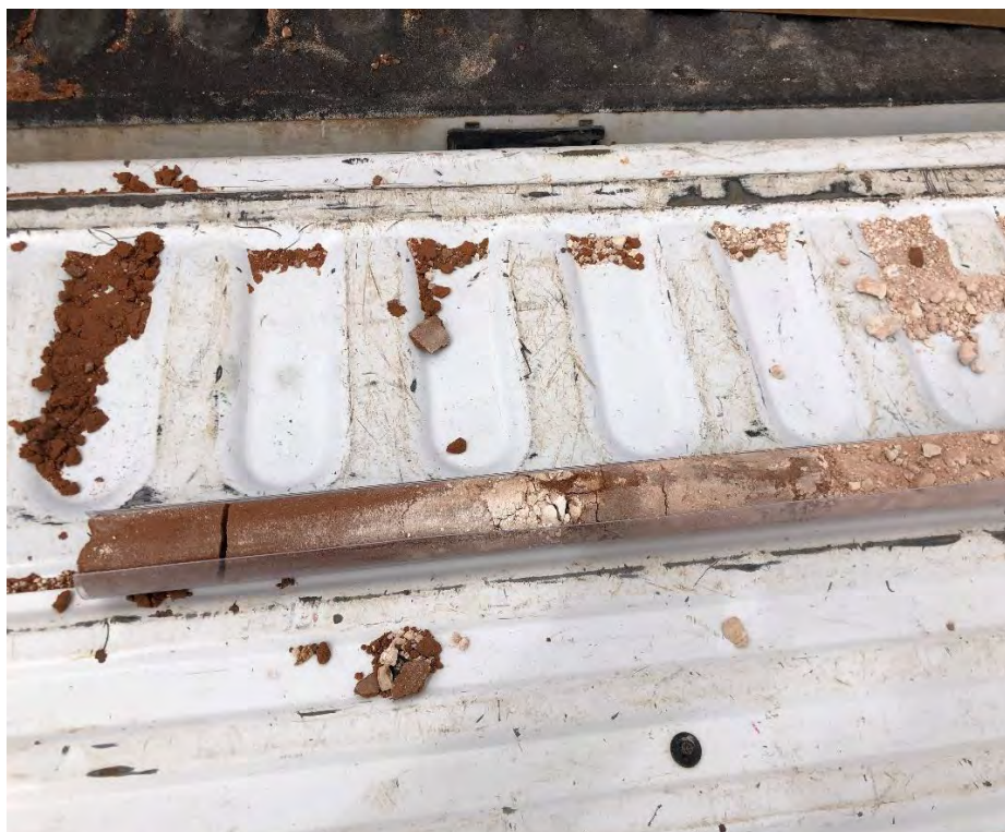
Photo 5. View of a Geoprobe sample core from 0 to 2 ft bgs
