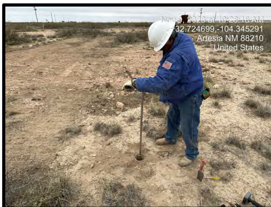
PHOTOGRAPH NO. 4 – A view of personnel installing a soil boring using a decontaminated hand auger to four feet bgs on November 9, 2023.
