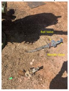
The following image depicts the new configuration to safely bleed down pressure from the intermediate casing, with multiple layers of protection including two ball valves, a choke valve and with the master valve dug out.
