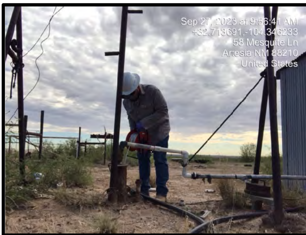
PHOTOGRAPH NO. 3 – A view of the water well depth-to-groundwater measurement collected by Ranger personnel.
