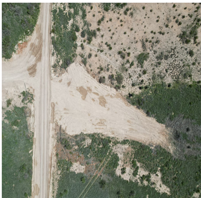
Aerial of Backfill to grade and lease road compacted.
