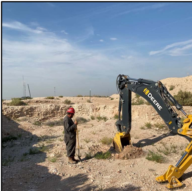
Photo 3: Advancing test pit at sample location B03. Note: Location is inside former pit, which is below the natural ground surface. Direction: Southwest
