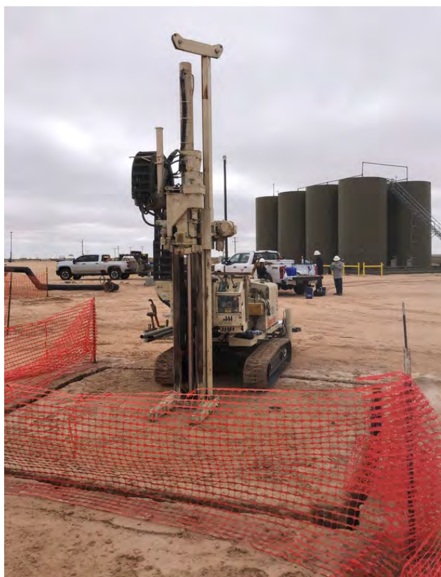
Figure 3: Sampling of GS-07 with a Geoprobe 6620DT, facing southwest.
