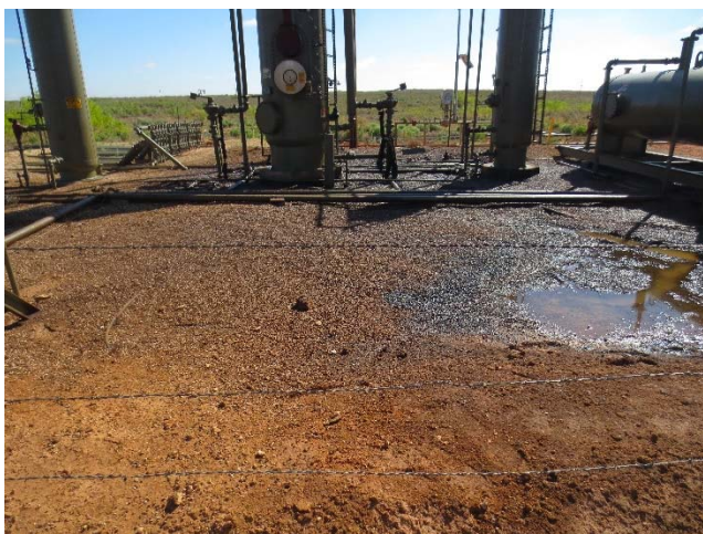
Standing Fluid inside berm SW corner
