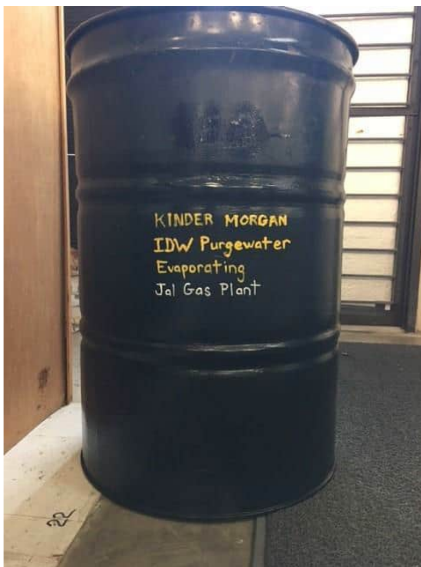
Jal #4 Gas Plant, Jal, New Mexico – IDW drum (coated inside & out, with Flex-Seal waterproofing protectant)
