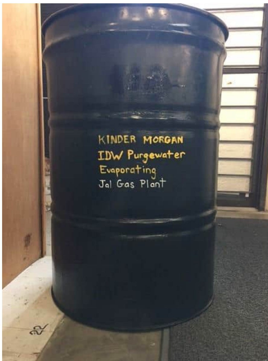
Jal #4 Gas Plant, Jal, New Mexico – IDW Drum Body, coated inside and out with Flex-Seal waterproofing protectant (to serve with Ventilated Barrel Cover)
