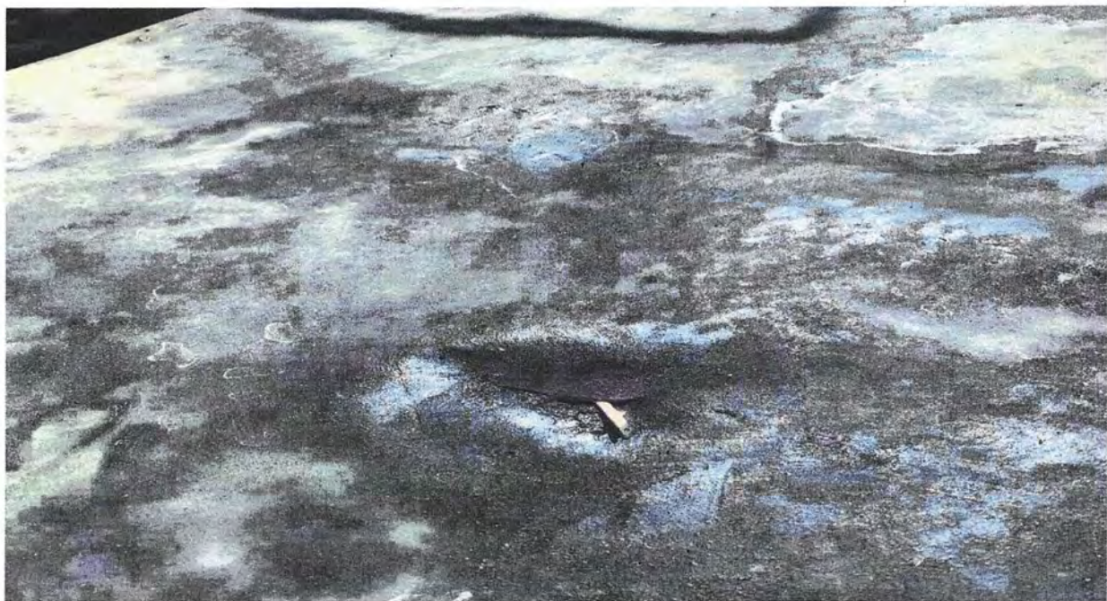
Small Mechanically Induced Hole in Liner – Designated Hole 2 - West Central Portion of North Side of the Lined Containment
