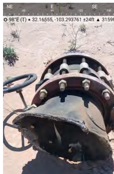
Figure 4: Damaged flowline that was severed in half that caused subject release.
