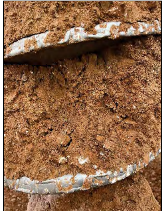
20-ft sample : Auger (left) and vitreous gypsum shown (bottom)
