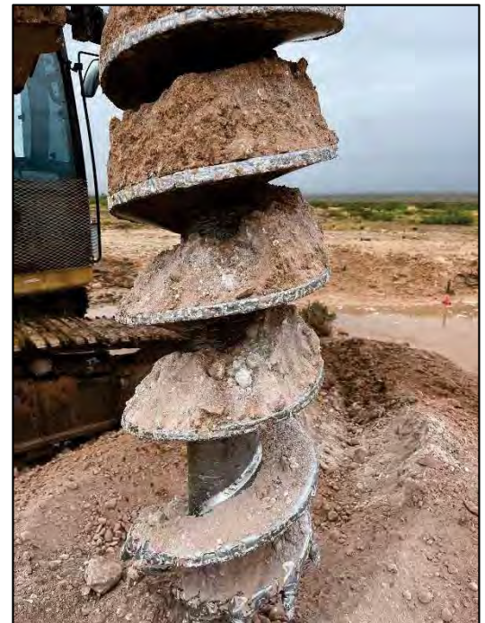
52-ft sample : hard limestone or dolomite in silt (left), auger(right)
