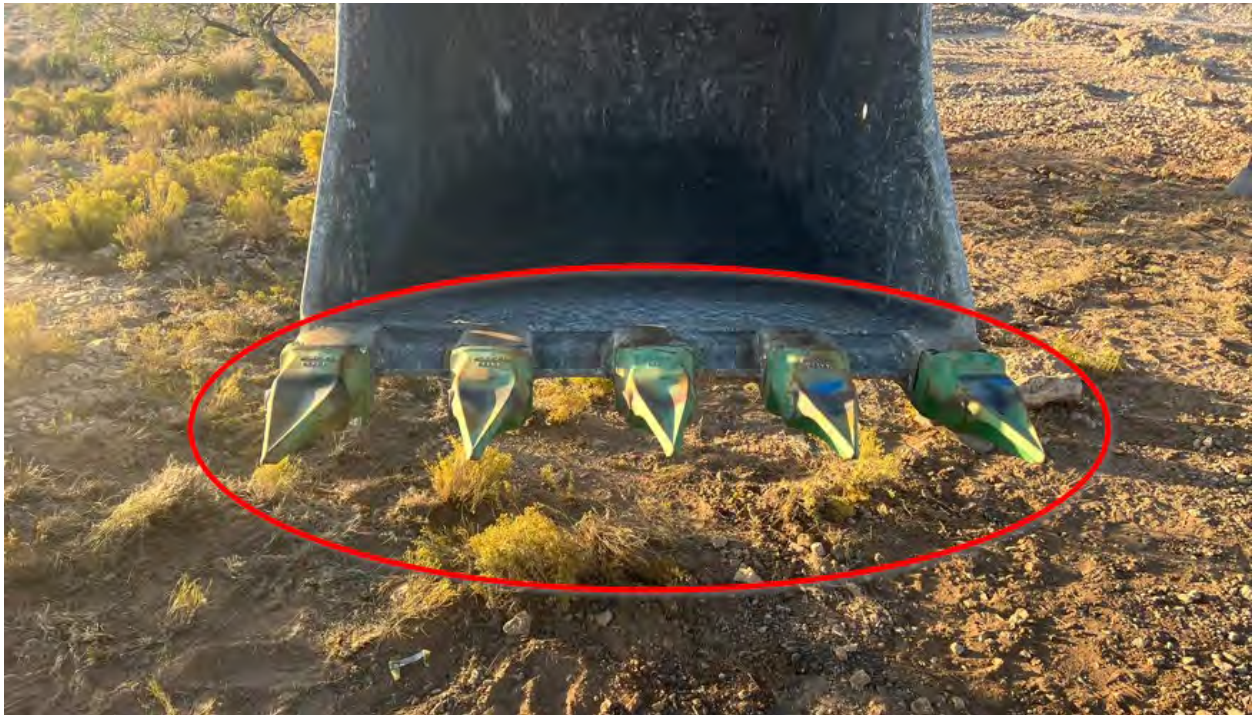
Figure 2: Sharks Teeth put on bucket of trackhoe to attempt to break through the hard caliche. October 11, 2024.
