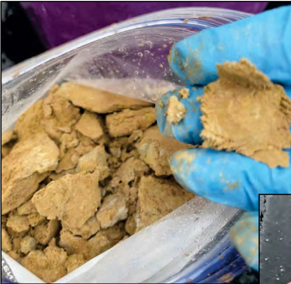
3-ft sample : demonstration of plasticity
