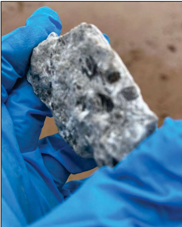
Hard dolomite or limestone at 95 ft
