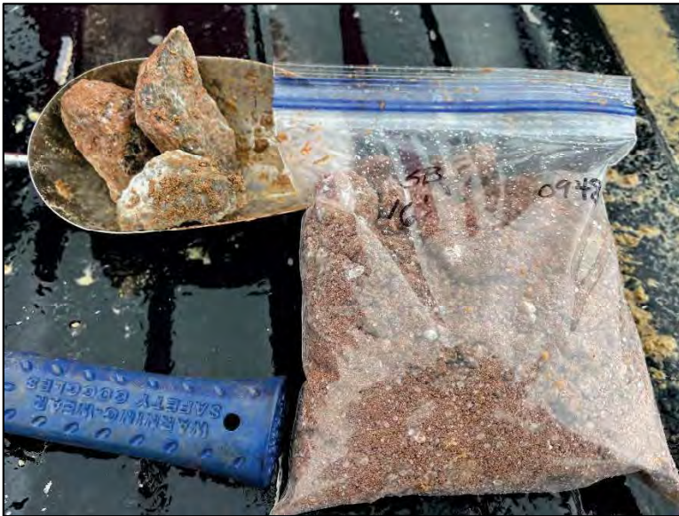
16-ft sample : Silt with gypsum or dolomite
