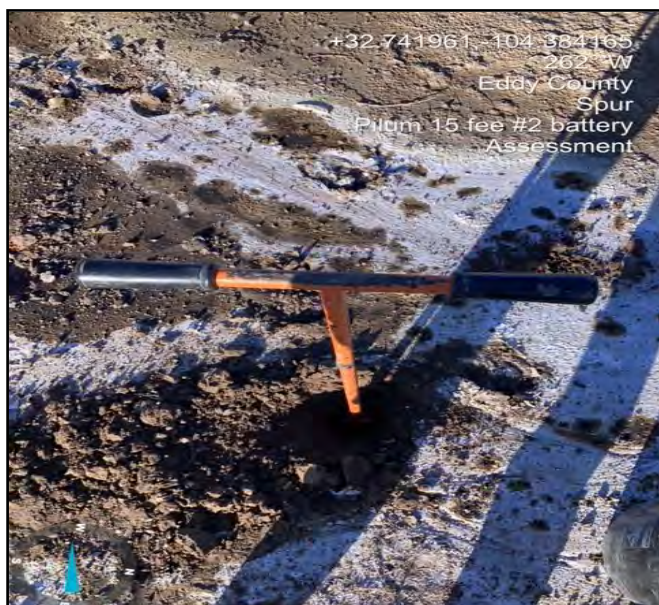
Photograph of a hand auger in the ground, facing West, to gather samples.
