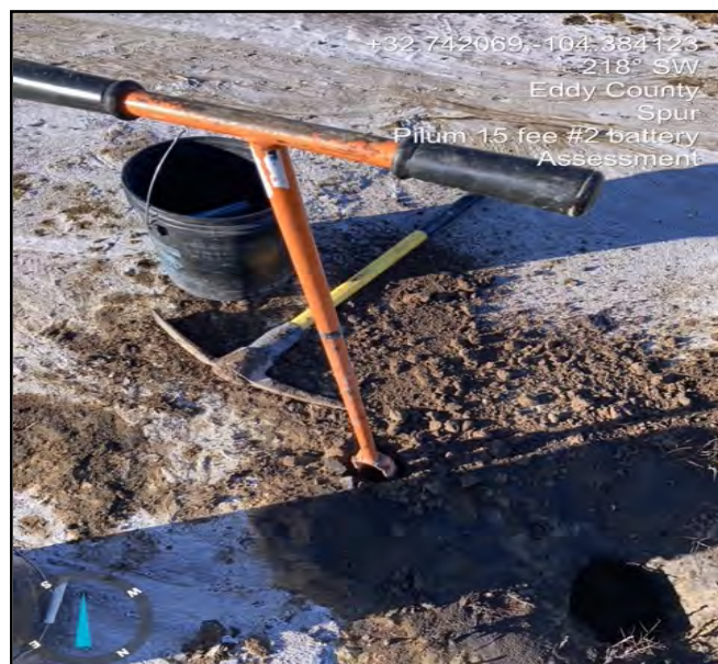
Photograph of a hand auger in the ground, facing Southwest, to gather samples.
