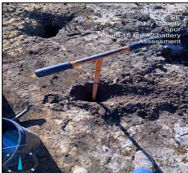
Photograph of a hand auger in the ground, facing Southeast, to gather samples.
