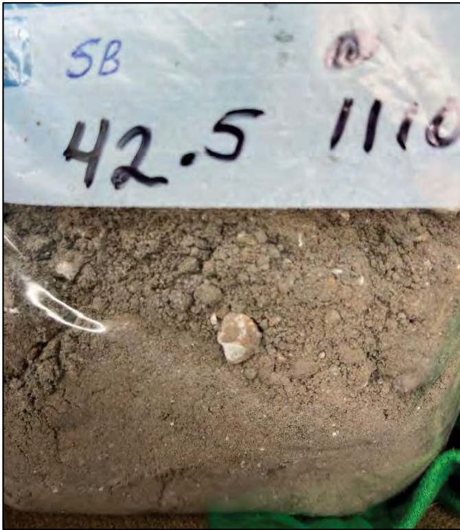
42.5 ft-sample : Silt with dolomite
