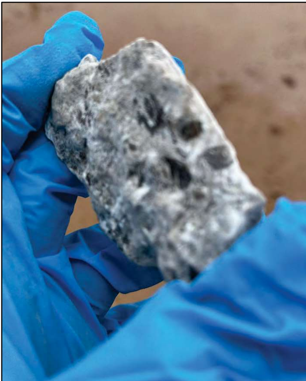
Hard dolomite or limestone at 95 ft
