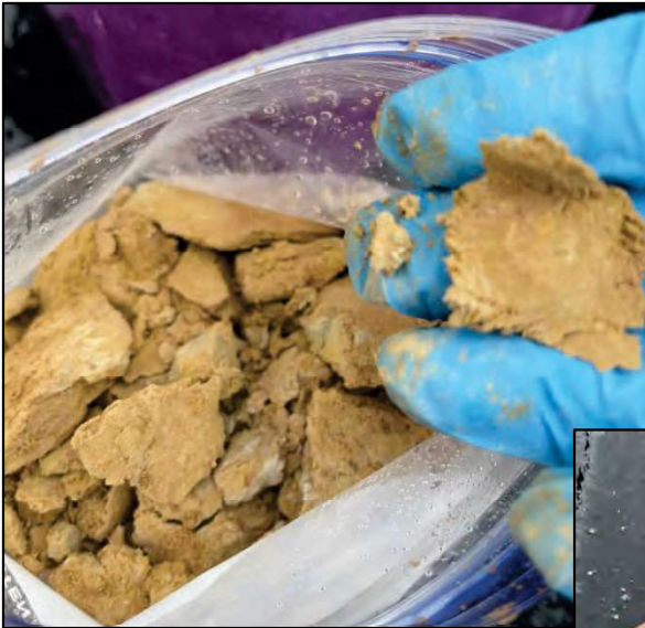
3-ft sample : demonstration of plasticity
