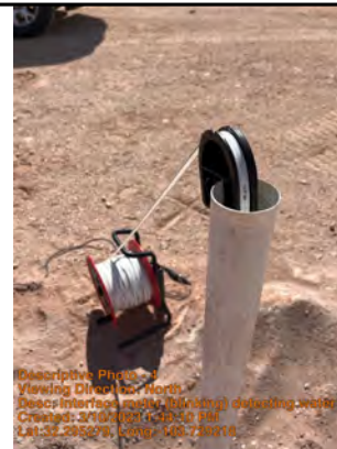
Interface meter (blinking) detecting water at measurement of 59 ft (with pipe)
