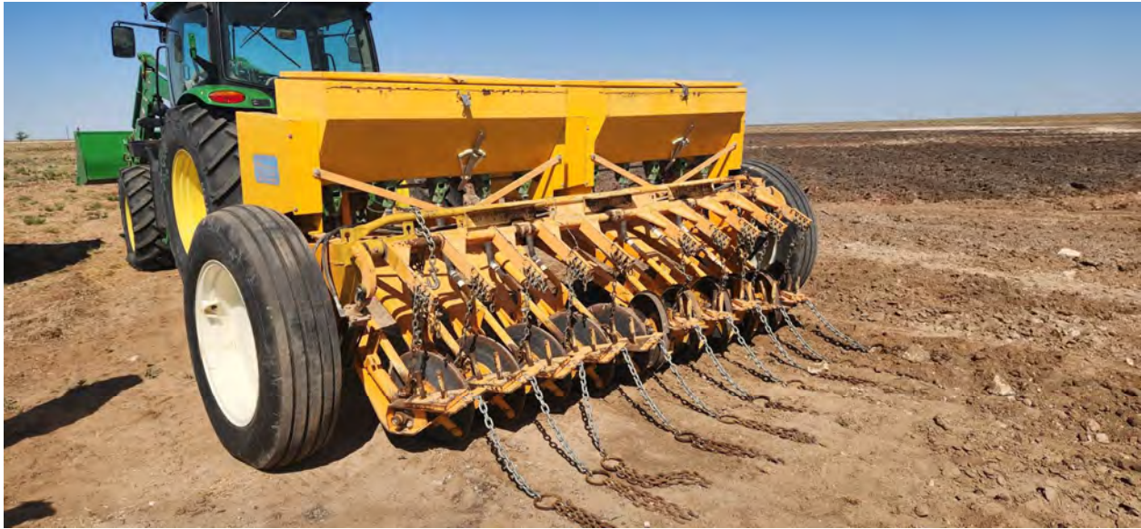
Photograph 37. Tractor-mounted seed drill used for kleingrass seeding. The seed is loaded in the hopper and dispersed at a calibrated rate; April 2025.
