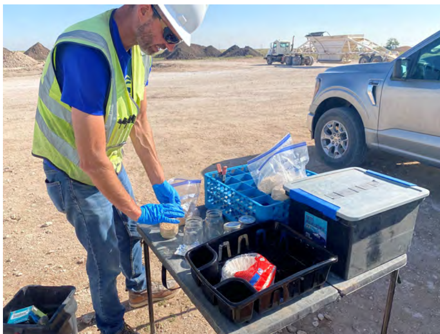
Photograph 9. INTERA geologist preparing samples for heated headspace analysis to screen for hydrocarbon vapors; April 2024.
