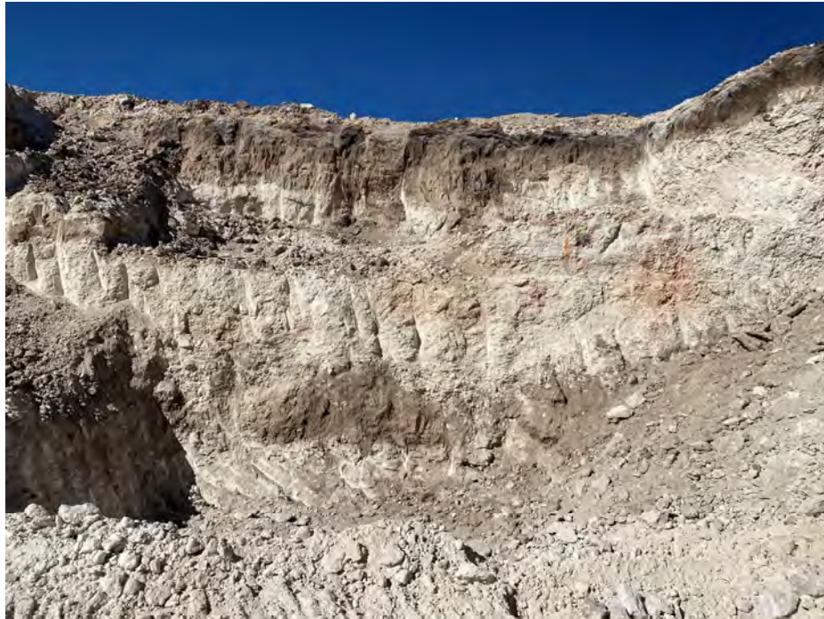
Photograph 7. Cross section showing both caliche and organic clay topsoil impacted by hydrocarbons; February 2024.
