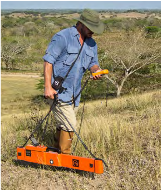
Exhibit 1: Measuring ECa with the EM38 in the vertical dipole position.
