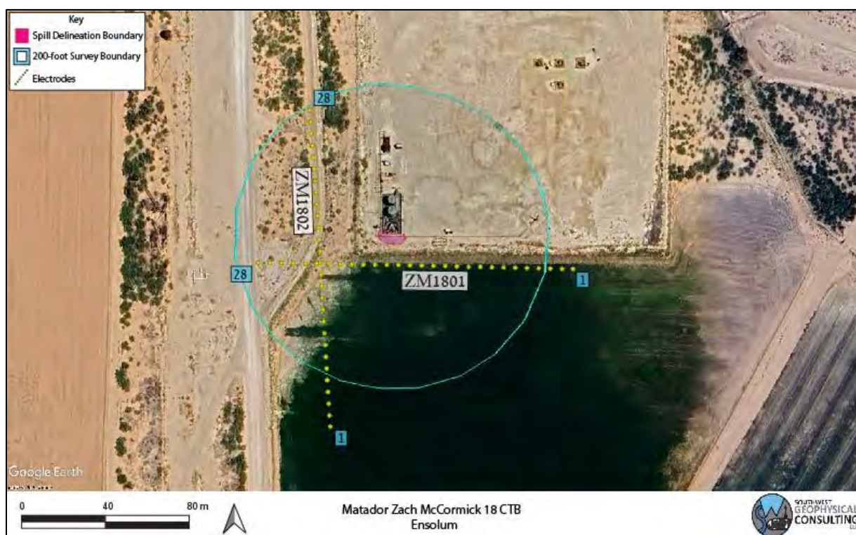
Figure 5: Geophysical survey overview. Two survey lines were conducted with 28 electrodes each at 5-meter spacing (yellow dots denoted with blue numbers). Background image credit: Google Earth. Image date: July 13, 2024. Image datum: WGS-84.
