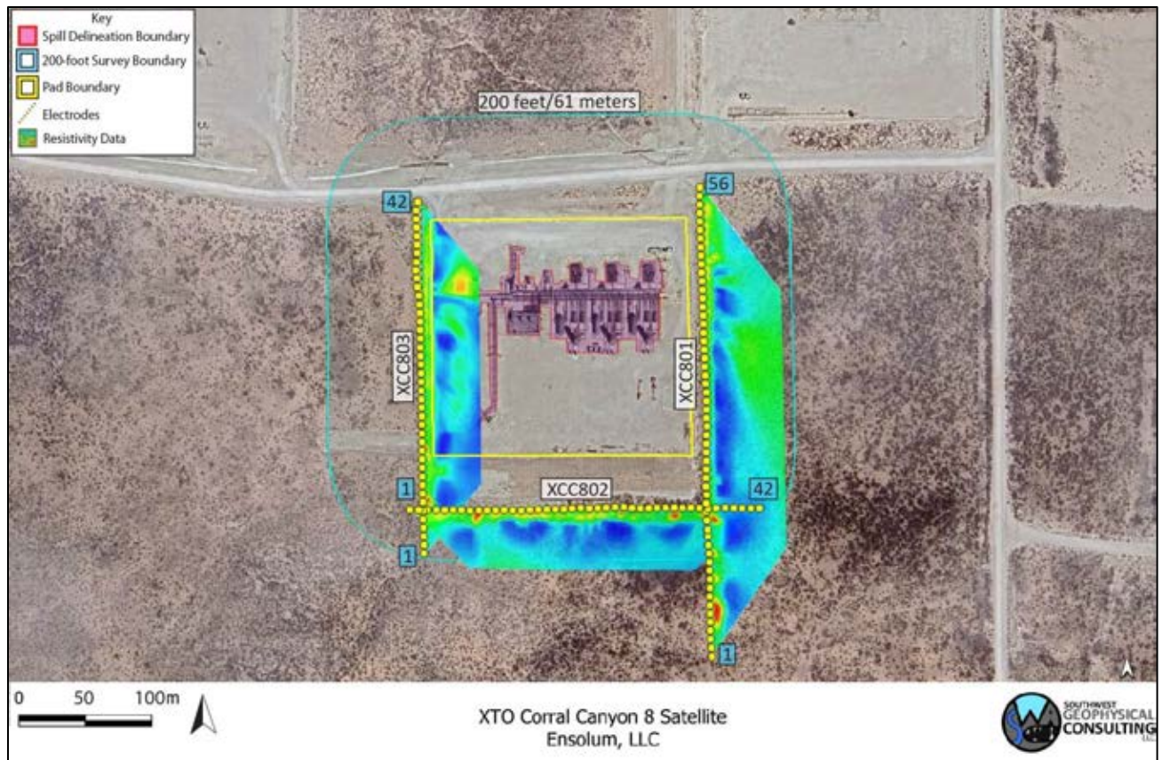
Figure 8: Data overlay. Colored trapezoids are 2D inverted resistivity lines. Background image credit: Google Earth. Image date: January 27, 2023.
