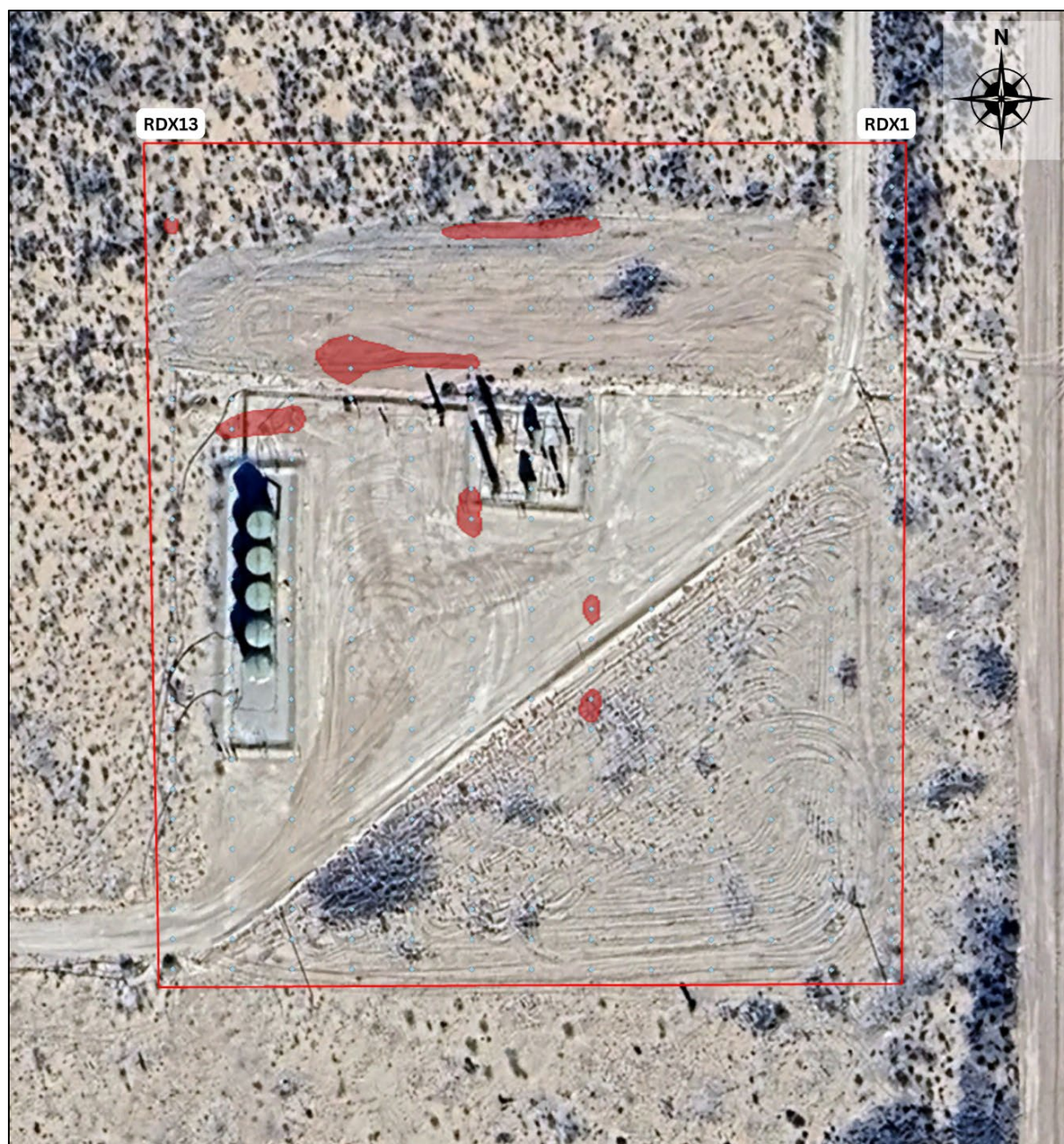
Figure A. Aerial view of the RDX 15 well pad illustrating the location of the subsurface anomalies delineated during the geophysical survey. These anomalies have been characterized as areas of increased porosity, air-filled voids and potential artifacts (false positives).
