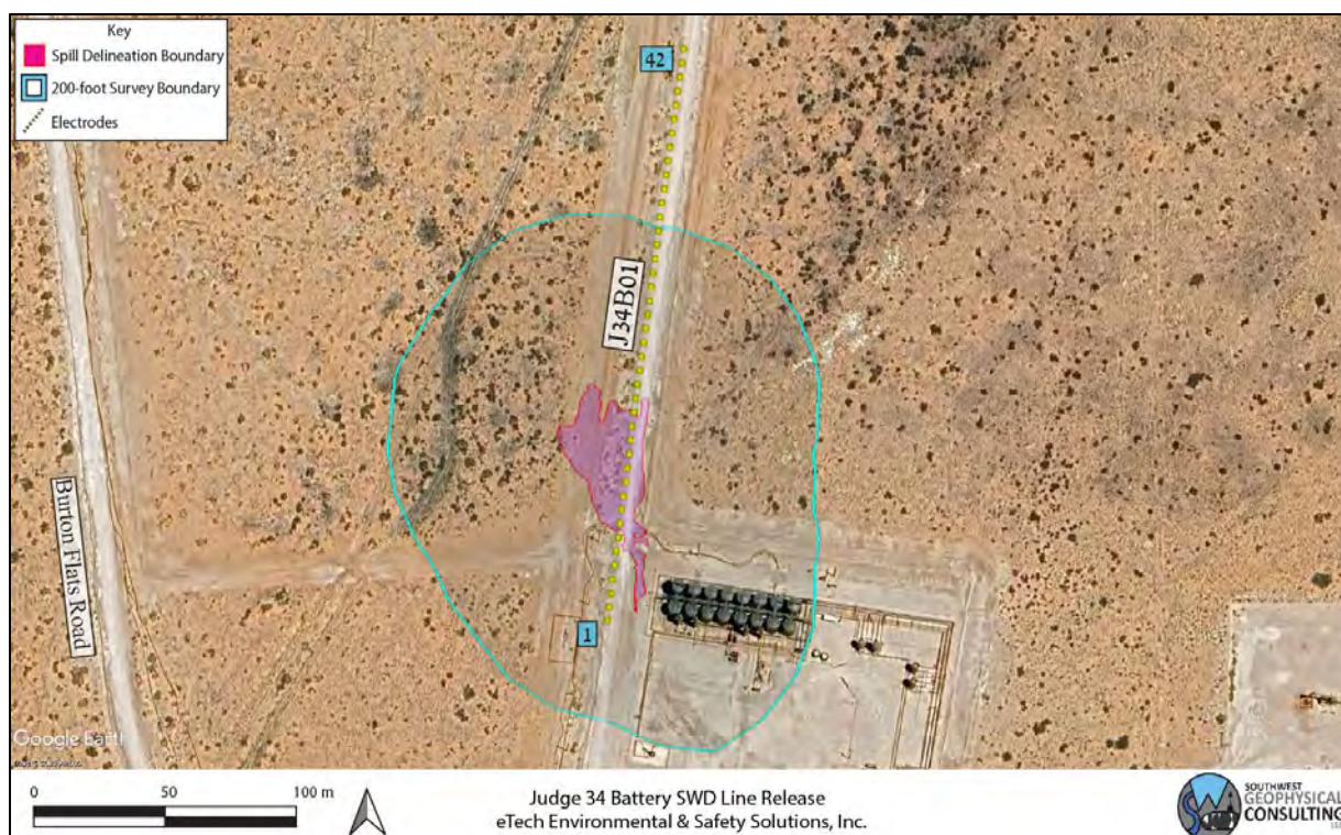
Figure 5: Geophysical survey overview. One survey line was conducted with 42 electrodes each at 5-meter spacing (yellow dots denoted with blue numbers). Background image credit: Google Earth. Image date: July 13, 2024. Image datum: WGS-84.
