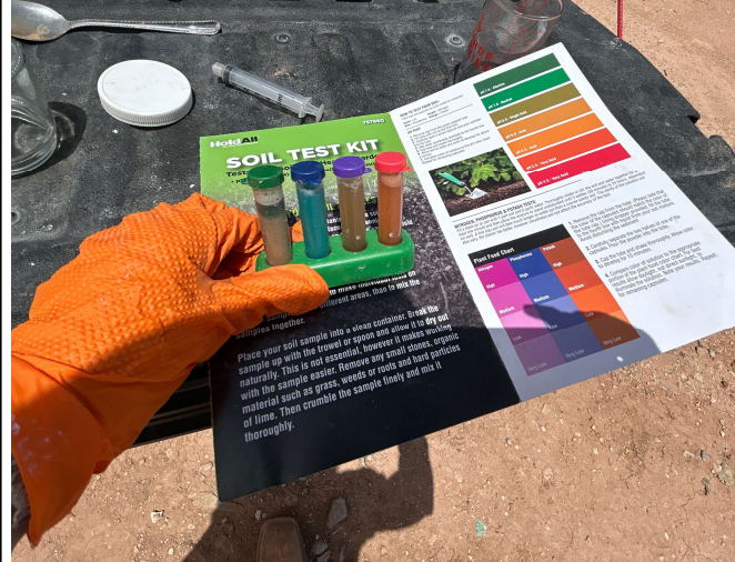
Photograph 3 Date: 05/29/2025 Description: View of nutrient sample testing of SC01.
