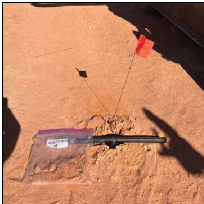
Photo 21. The CS-03-CB soil sample was collected via hand-auger from approximately four feet below ground surface (4 ft bgs).
