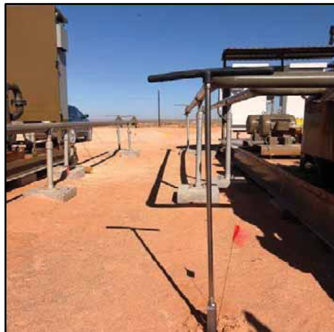
Photo 23. View of CS-04-CB sample location. The four foot hand-auger used to collect both CS-03-CB and CS-04-CB soil samples is shown in the foreground.
