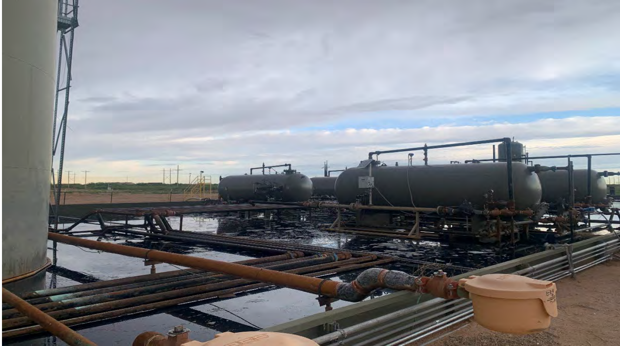
Photo 3: May 15, 2025 view showing fluid retention and poly metal berm integrity.
