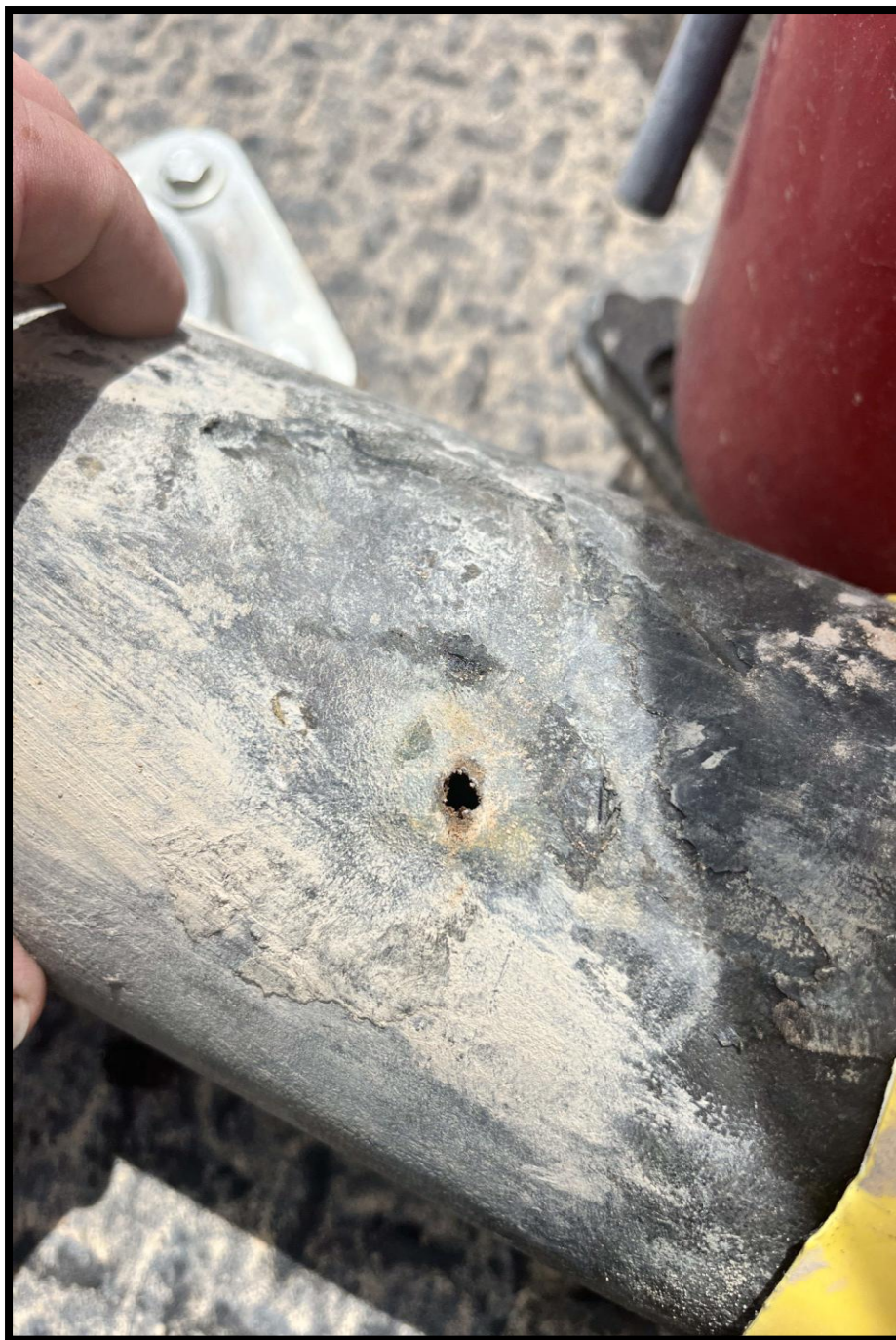
Photo 3: Pin hole in pipeline that caused the release.
