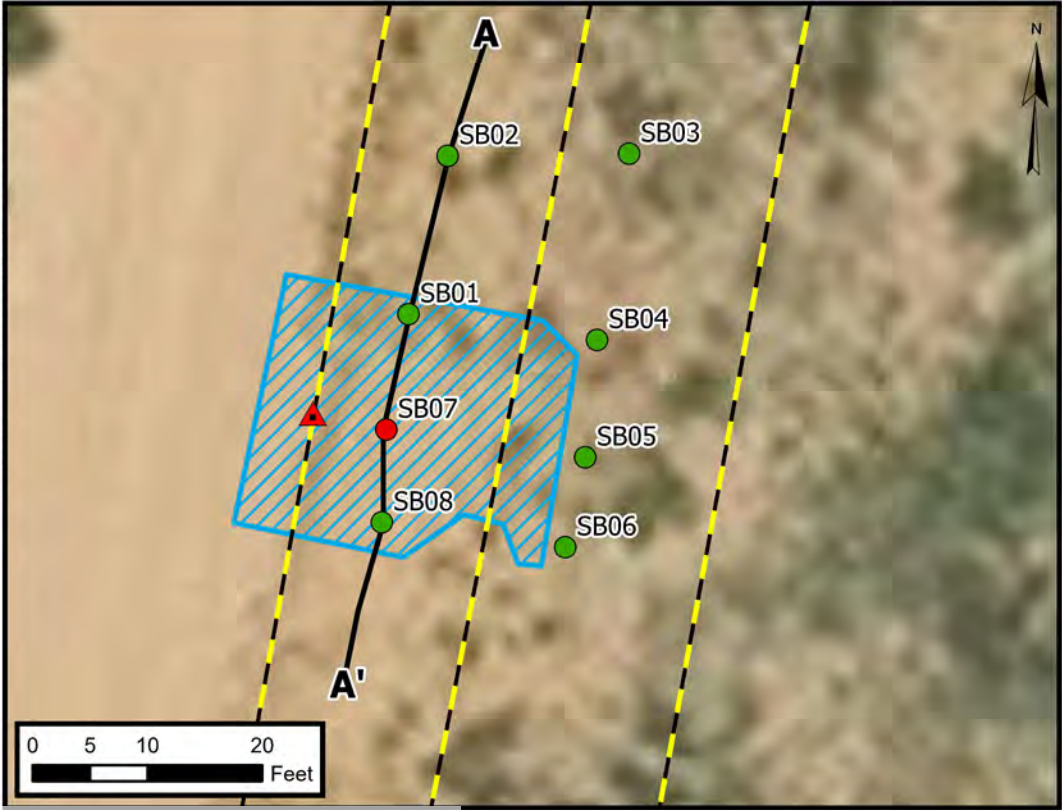
Cross Section A-A' with Interpolated TPH Plume Enterprise Field Services, LLC Blanco C-7 (January 2025) Unit A S14 T26N R9W San Juan County, New Mexico 36.49199, -107.75149
