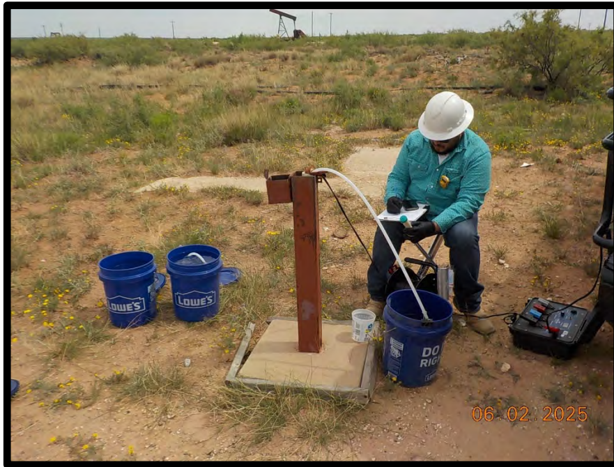
PHOTOGRAPH NO. 1 – A general view of the low-flow sampling methodology during the June 22, 2025 monitoring event.
