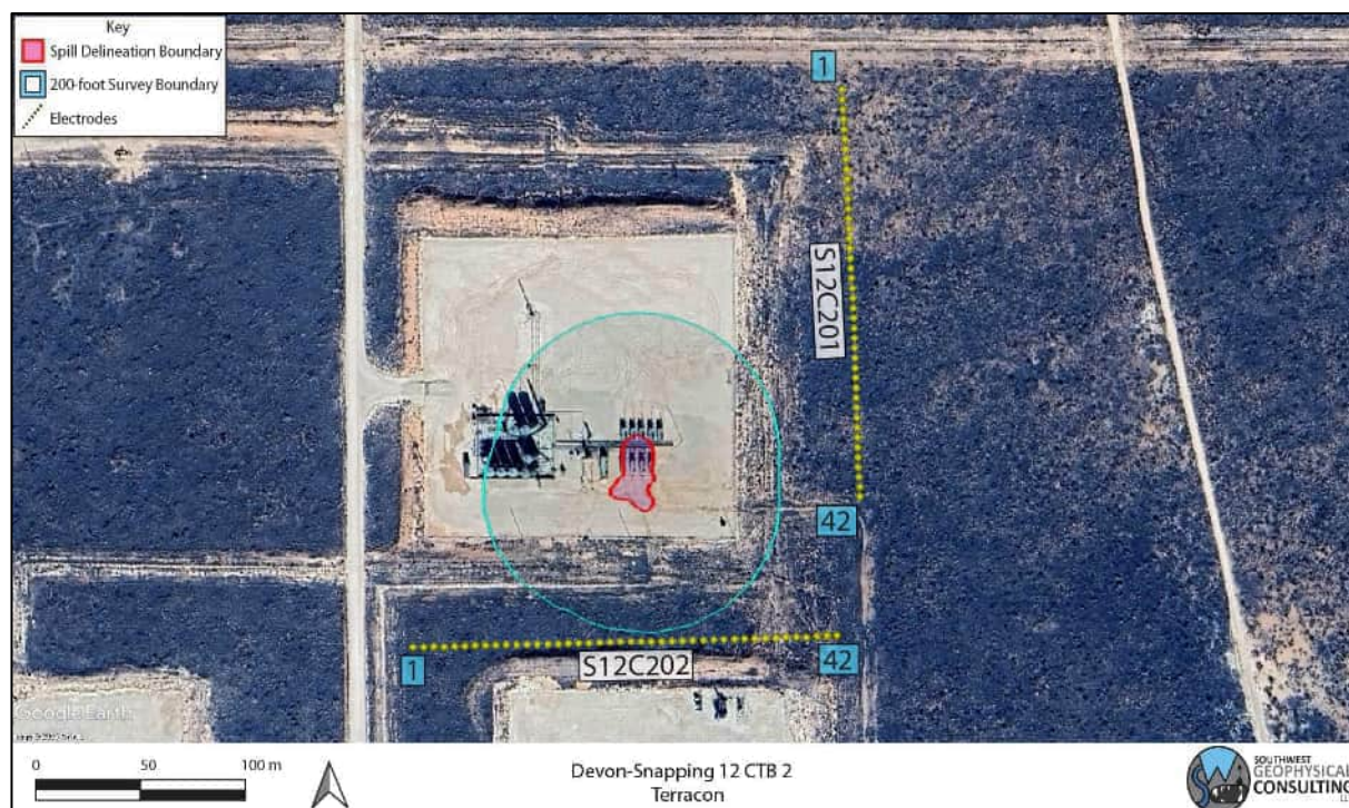
Figure 5: Geophysical survey overview. Two survey lines were conducted with 42 electrodes at 5-meter spacing (yellow dots denoted with blue numbers). Background image credit: Google Earth. Image date: December 20, 2023. Datum: WGS-84.
