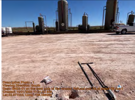
BH25-01 on the west side of the release. Refusal was hit at about 1ft due to a highly compacted sand layer
