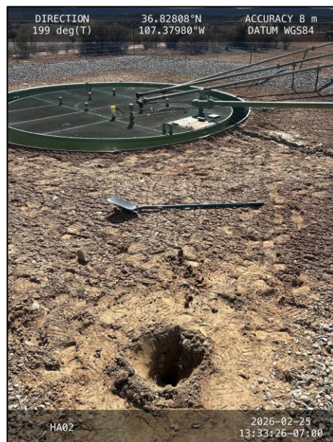
Photograph: 3 Date: 02/25/2026 Description: Hand auger boring HA02, advanced to the north of the source of the release. View: South
