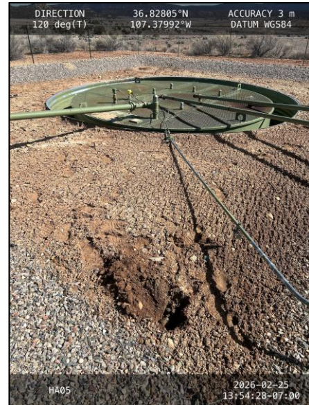
Photograph: 6 Date: 02/25/2026 Description: Hand auger boring HA05, advanced to the west of the source of the release. View: Southeast
