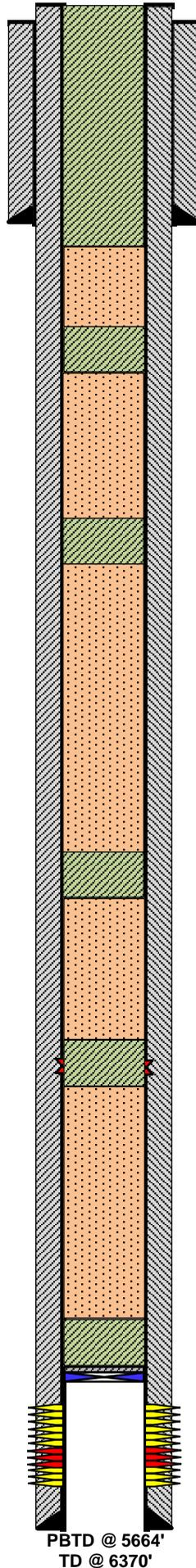
6. PUH & spot 65 sx Class "C" cmt from 650' to surf, fill up. (Surf Shoe, Water Board, & Surf Plug)
