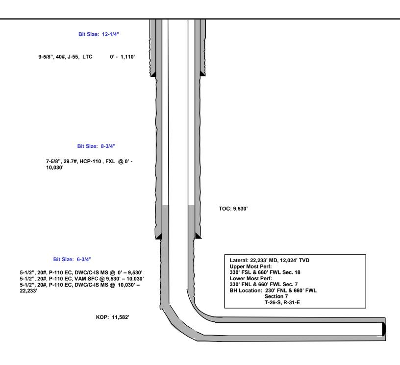
912' FSL 893' FWL Section 18 T-26-S, R-31-E Proposed Wellbore Design B KB: 3,210' GL: 3,185'
