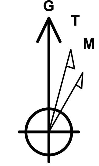
Azimuths to Grid North True North: 0.64° Magnetic North: 9.33°
