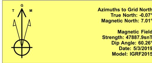
To convert a Magnetic Direction to a Grid Direction, Add 7.01°
