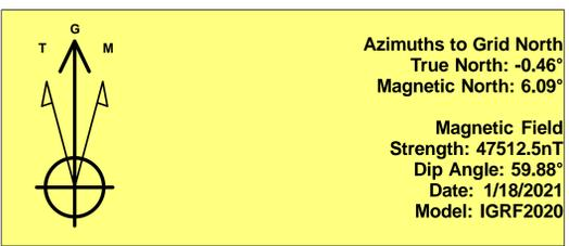
To convert a Magnetic Direction to a Grid Direction, Add 6.09°
