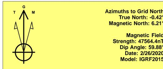
To convert a Magnetic Direction to a Grid Direction, Add 6.21°
