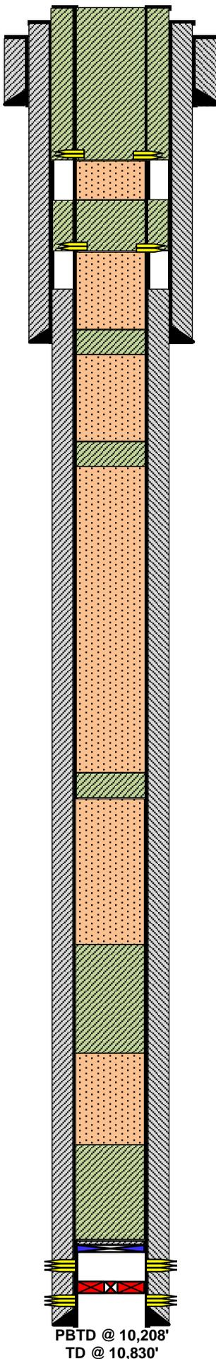
7. PUH & perf'd @ 900', broke CIRC & sqz/CIRC 300 sx Class "C" cmt from 900' to surf. CIRC 5 1/2" to surf. RDMO, cut off WH, install dry hole marker & clean location.(7 Rvrs, Yates, Water Board, & Surf Plug)
