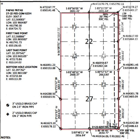
1. BEARINGS SHOWN ARE GRID BASED ON THE NEW MEXICO STATE PLANE EAST ZONE COORDINATE SYSTEM (3001), NAD 83 (2011), BASED FROM GPS OBSERVATIONS, OCCUPYING A WHS CONTROL POINT (5/8" REBAR), LOCATED AT NORTH: 456034.443, EAST: 653560.64 LELEVATION: 3101.373, DETERMINED BY AN OPUS SOLUTION ON DECEMBER 3RD, 2018.
